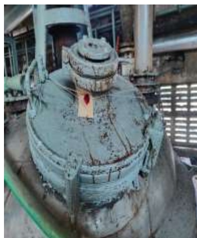
Manhole (material charging hole) of total 6 nos. of reaction vessels provided in production plant area of the units are sealed
