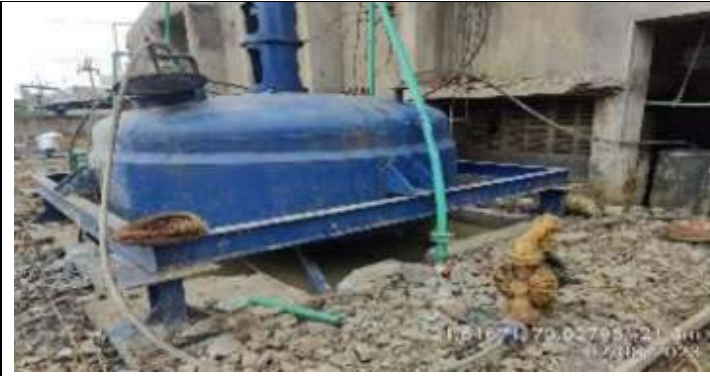
Material was transferred by AOD Pump connected with Separator Vessel and a flexible pipeline open at ETP
