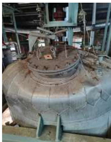
Manhole (material charging hole) of total 6 nos. of reaction vessels provided in production plant area of the units are sealed
