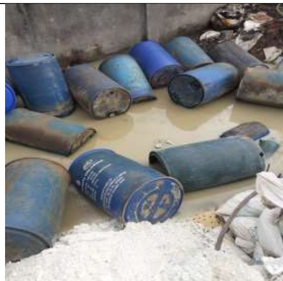
Alkaline (@ 10 pH on pH strip) containing w/w is being leach out from the stock of Haz. Waste and hence ponding of alkaline w/w is created on kuchcha land within premises.
