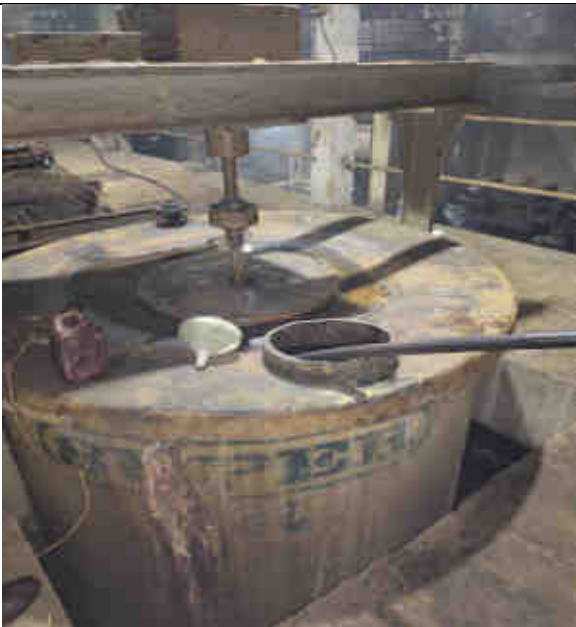
Flexible pipeline with pump from reaction vessel to final treated w/w holding cum CTEP disposal tank
