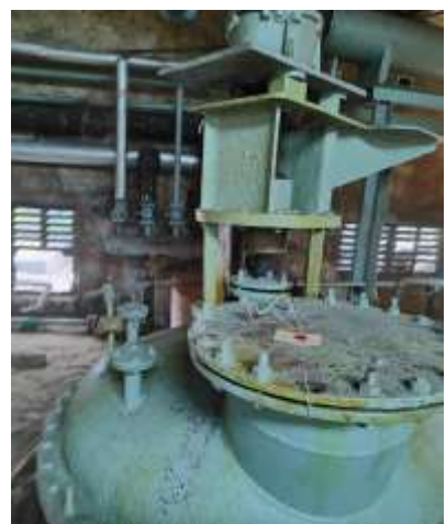
Manhole (material charging hole) of total 6 nos. of reaction vessels provided in production plant area of the units are sealed
